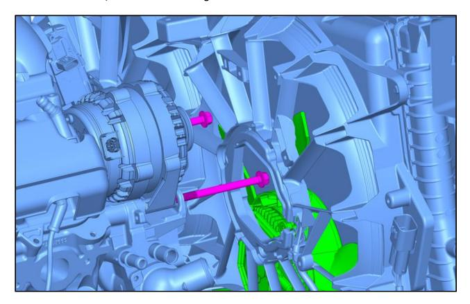
**Note:** The passenger side alternator bolt is very long and will interfere with the fan motor upon removal. Disconnect the wire connector, remove the fan motor's perimeter bolts, and carefully position the fan assembly out of the way inside the shroud. Be careful not to let the fan contact the radiator or damage could occur.
