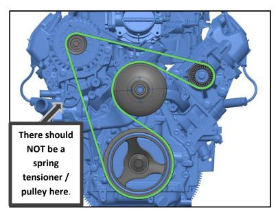
**Pulley note:** This alternator is specifically designed to work with GM truck's original stretch fit belt. Changing the pulley diameter would impact the required belt length. Only the supplied Mechman pulley should be used.
