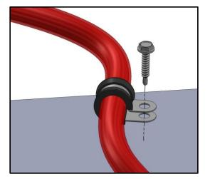
Use screws and insulated mounting clamps (not included) to secure larger cables to the vehicle.
