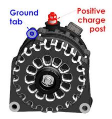
11. Upgrading the alternator grounds: The ground boss tab on the rear alternator housing ABSOLUTELY must be used. Anodized billet alternators are non-conductive internally. A 1/0-gauge ground cable MUST be run from the alternator ground tab, directly to the negative terminal of the battery. Failure to do so will cause damage to the alternator and cause potential harm to other components.
