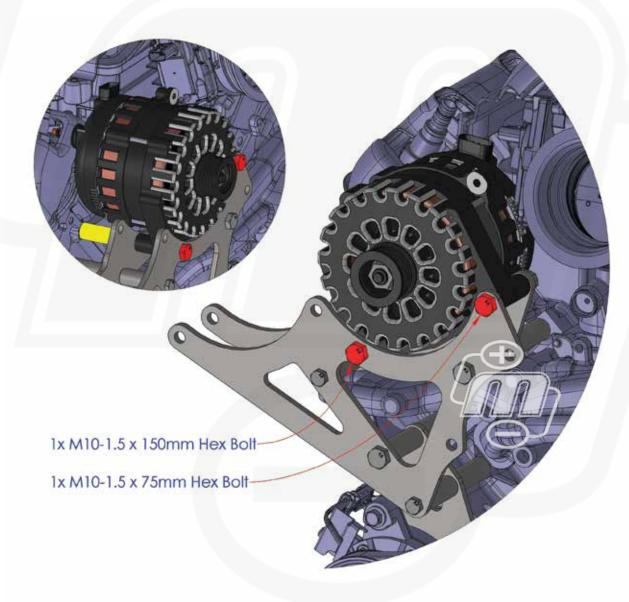
**Step 5:** Install the second OEM Compatible Alternator
