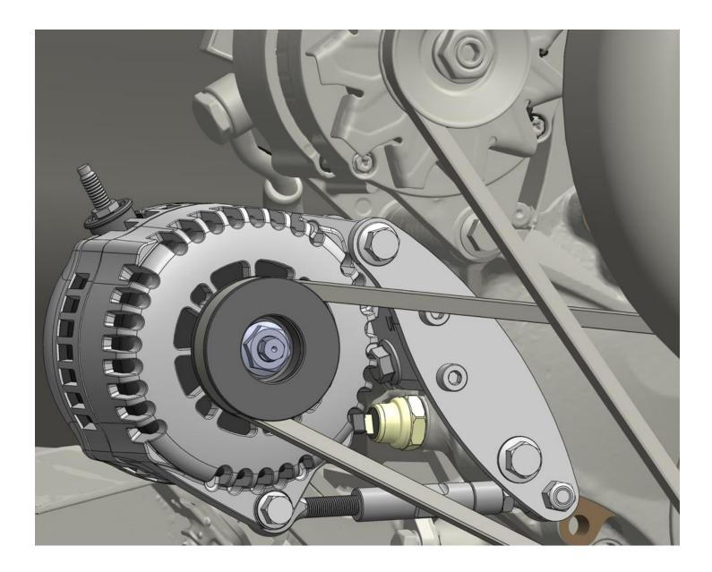
Wiring: a dedicated 4-gauge positive and ground must be run directly from the alternator to the battery.
