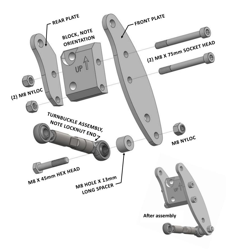
7. Install the bracket assembly to the engine block.
