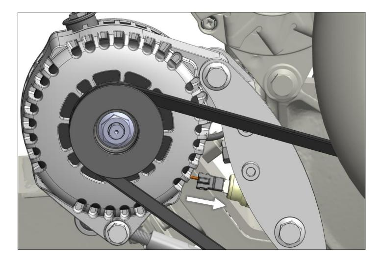
13. Confirm the original alternator spacer tab is rotated so that it is not interfering with the second alternator bracket OR the back of the engine block. Center the tab between the engine block and alternator bracket.
