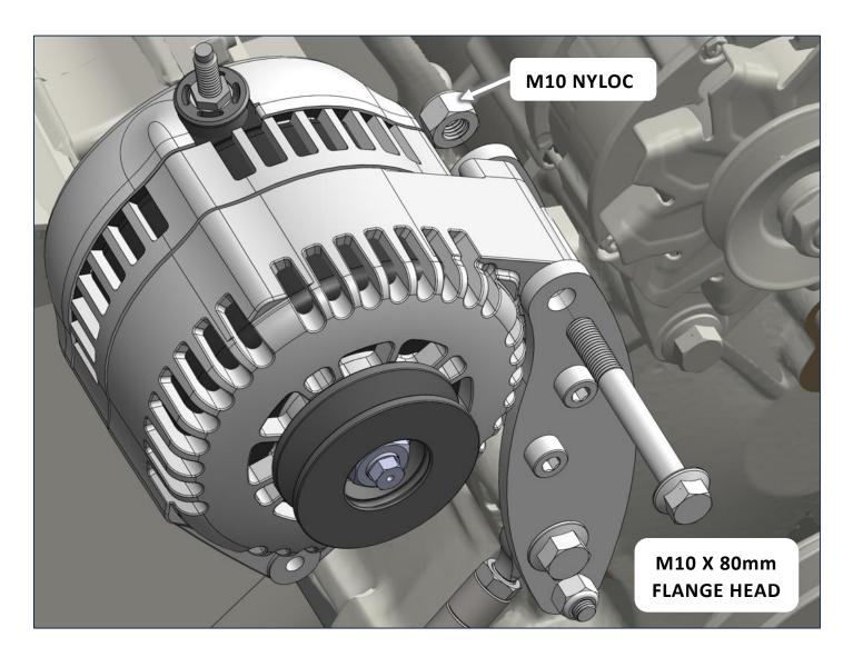
9. Loosely install the supplied belt over alternator and crank pulleys at this point.
