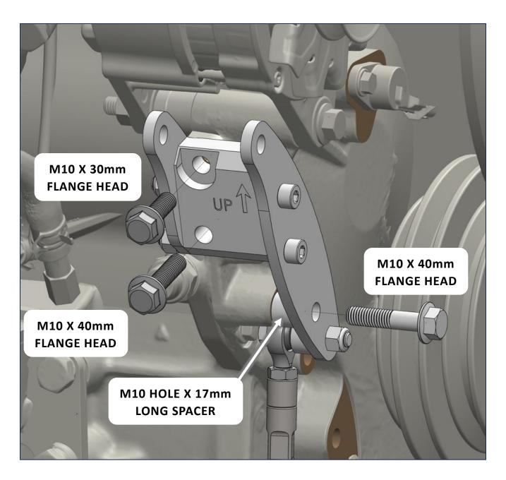
8. Install the alternator's main mount to the bracket assembly. Snug tight, but where alternator will still swing when pushed.
