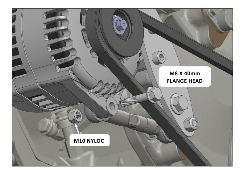
11. Tighten belt with turnbuckle and belt (do not over tighten). Once tight, hold the turnbuckle shaft with a wrench and tighten the jam nut.
