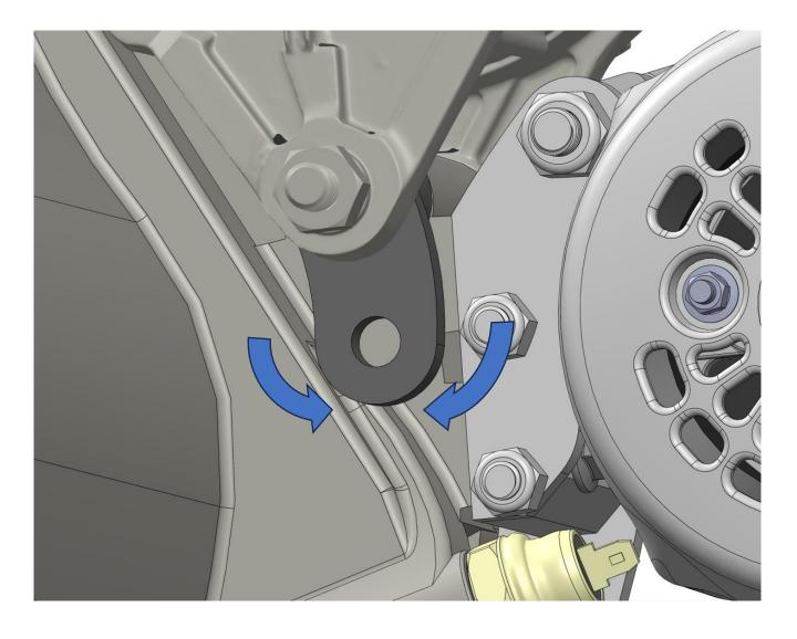
14. Install the original belt. Tighten the original alternator tensioner until that belt is tight (do not over tighten). Snug that tensioner's jam nut.
