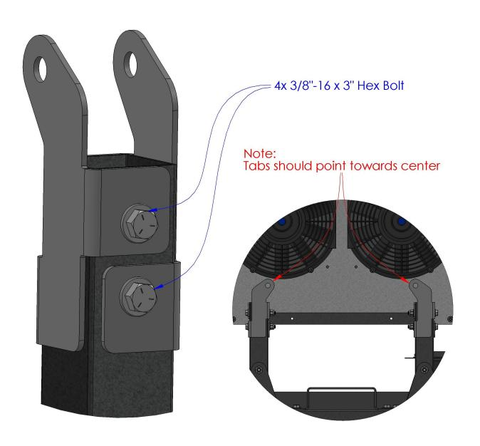
**Step 2:** Attaching the 2WD Transmission Mount to the Rear Engine Mount Bracket
